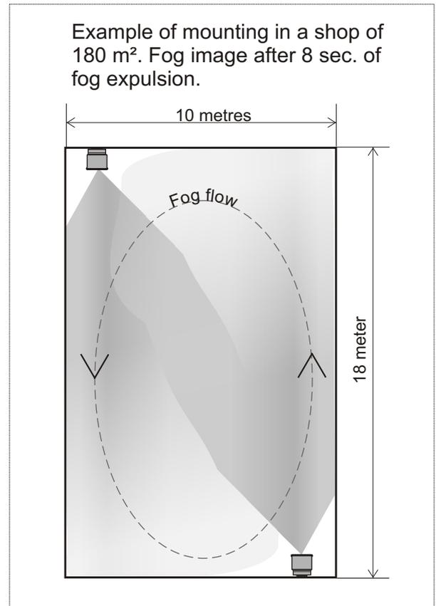
The **BANDIT 240** has a room filling capacity of ~28 m<sup>3</sup> per second. This corresponds with ~10 m<sup>2</sup>/sec. The max. surface area which can be secured with one device is equal to the max. fog expulsion period = 18 s x 10m<sup>2</sup>/s which is 180 m<sup>2</sup>. For larger surfaces, such as: large shops and office spaces, one has to install more devices, one device each 170 m<sup>2</sup>
